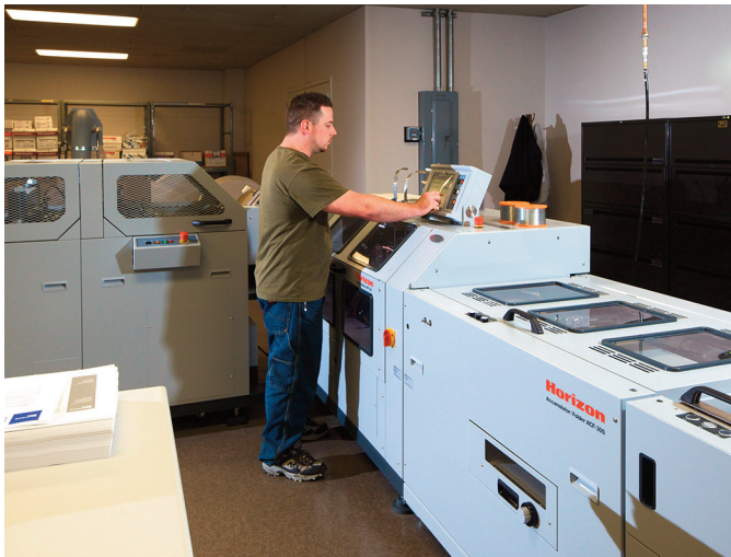
Unwinding and cutting technology from Hunkeler enables highly efficient in-line production on the Horizon StitchLiner 6000 Digital at speeds up to 6,000 booklets per hour.
