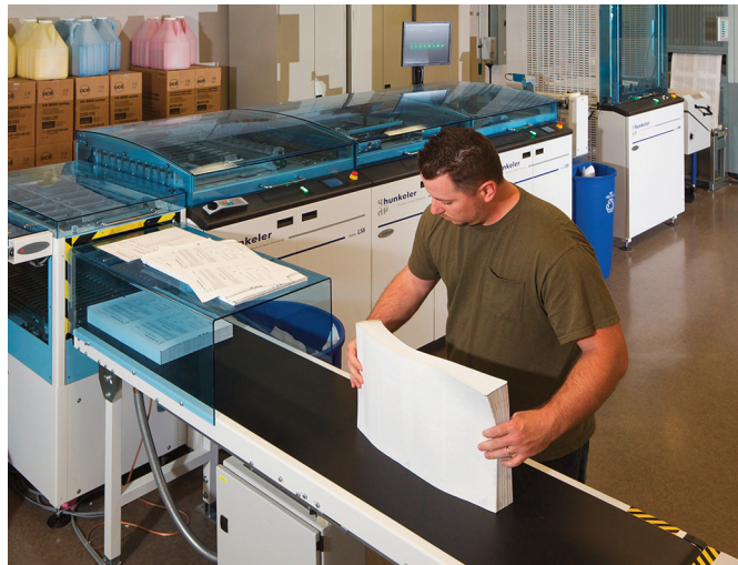
The in-line digital finishing solution has been customized as a Roll-to-Booklet/Roll-to-Stack combi line for saddlestitched booklets, straight stacks or separated book blocks as needed.
