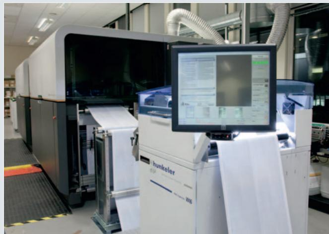
The WI6 web inspection system is integrated into the production line following the Kodak VL4200 printer. The monitor shows the image captured by the cameras at every point in time. Possible errors can then be quickly identified by the operator.
