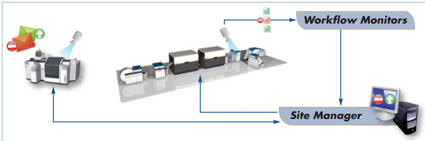
**The DVLA currently examines the printed paper web with high-resolution cameras. Bad printed images are recognised, and the affected copies are diverted. With the planned expansion to a closed-loop system, the DVLA will soon have at its disposal comprehensive functions for monitoring quality and process analysis.**
