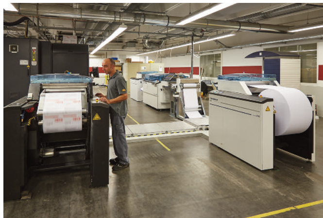
Due to the tight time frames involved, preference was given to inline production at SPS. Alternatively, the parallel production of different jobs in offline mode is also possible.
