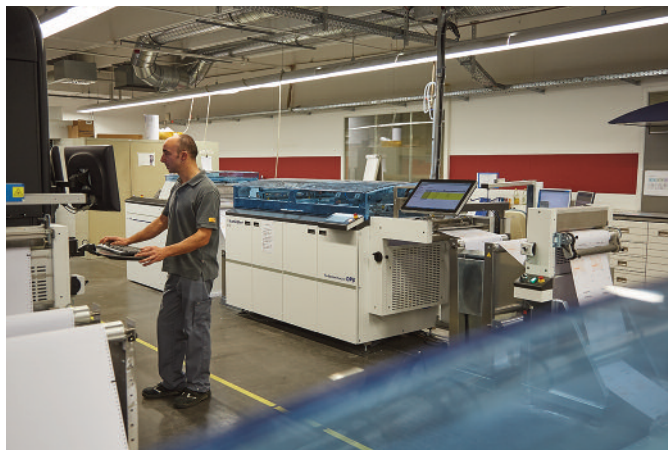
The DP8 modules can produce documents with variable content and dynamically changing punching and perforation templates – from the white paper web right up to the end product.
