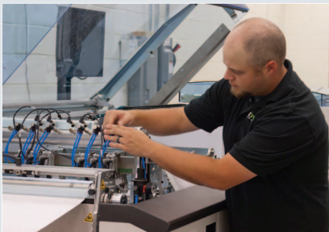
The DP6 Dynamic Perforation Module allows Mail Print to produce personalized coupons for use at entertainment venues where perforating accuracy is critical to facilitate efficient redemption.
