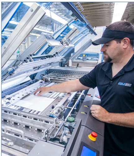
An EBSCO Media technician makes final adjustments to the Hunkeler Cut/Stack system before running the next job...
