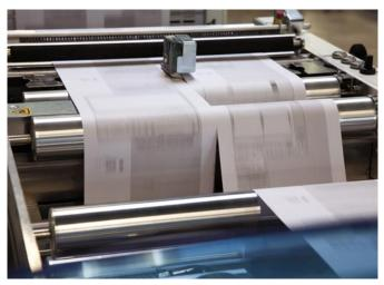
A key component in the POPP6 line is the web merger WM6. Following the slitter section, the two paper webs are precisely superimposed before they enter the CS6 cross cutter.
