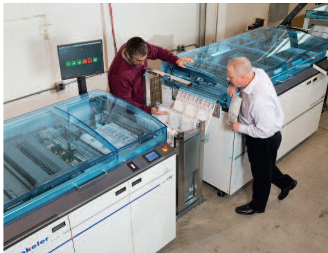
On a DP8-II Dynamic Perforating Module (on the right) the individual pages are being enhanced dynamically with variable perforating patterns, both lengthwise and crosswise.
