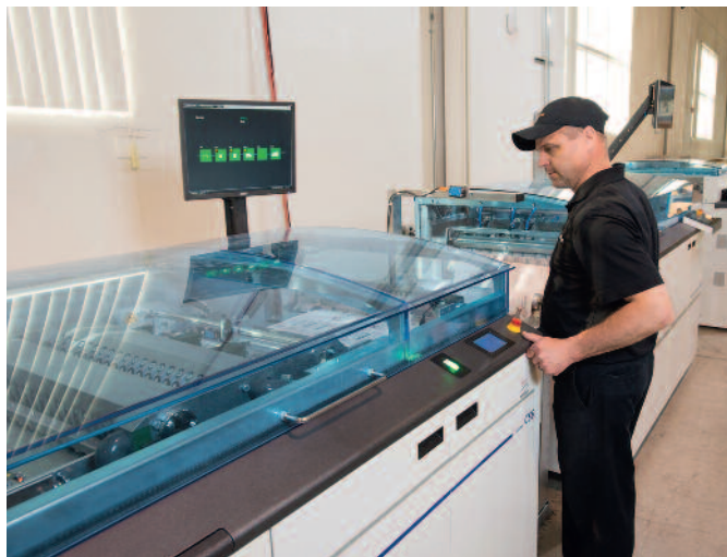
Heeter has decoupled the finishing process from printing. The printed web is processed near-line to block blocks on a Roll-to-Stack system from Hunkeler.
