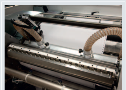
The PP6 punching and perforating module is a crucial component that leads to economic operation and value-added in the DVLA production lines. The ability to add guide holes and fold perforations (the perforating cylinder is shown in the picture) is integrated into the same module. The in-line process makes it possible for the DVLA for the first time to dispense with externally prepared rolls of full colour pre-printed documents and instead produce them in-house on the two Hunkeler lines.
