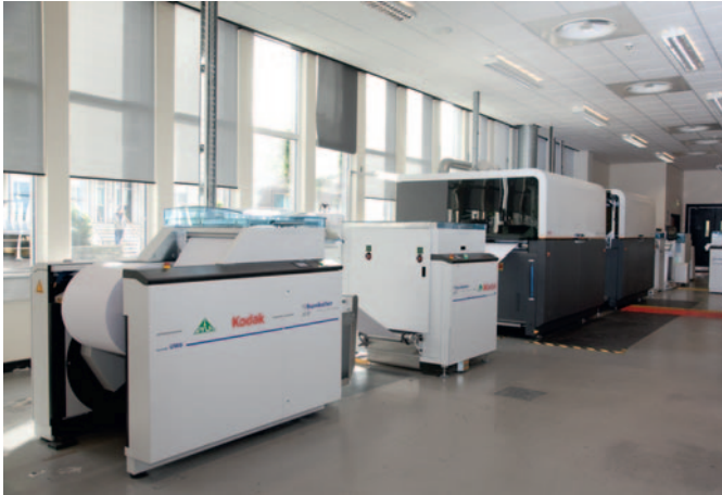
Thanks to the PP6 (middle of the picture), starting with white rolls the DVLA has increased production volume now done in-house by between 50 and 60 million documents per year.
