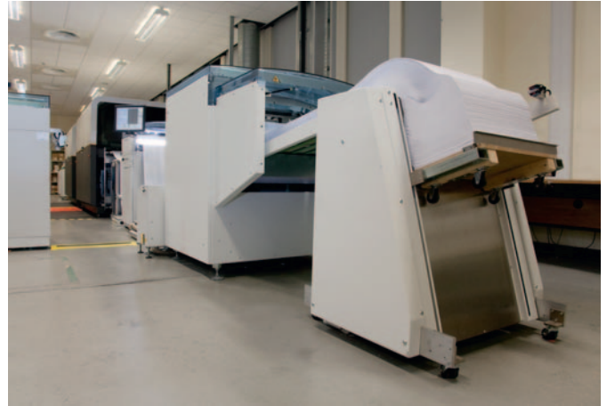
With stacks reaching 700 mm, the FF6 folder stacker achieves the excellent quality that is the pre-requisite for a noticeable jump in productivity during insertion.
