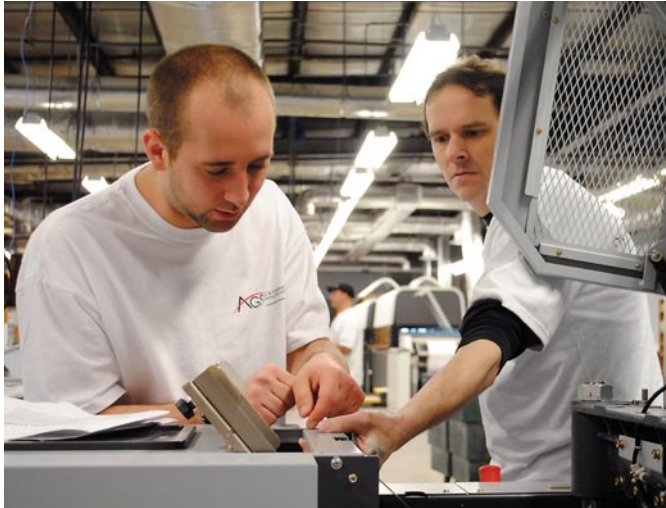
Tommy Greene and Mike Schaffer make final adjustments to the StitchLiner 6000 Digital at AGS. Preprinted rolls are converted to cut sheets and then booklets in a single pass with no touch points.
