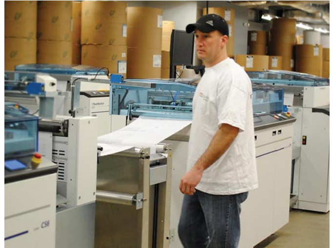
Joe Dziedzic is AGS Lead Digital Production Specialist. He monitors the finishing requirements of a customer booklet through the Hunkeler CS6 cutter.
