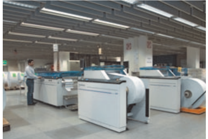
The offline lines for roll-stack production recognize the codings of the different envelope production systems. The client gains a high degree of processing flexibility.
