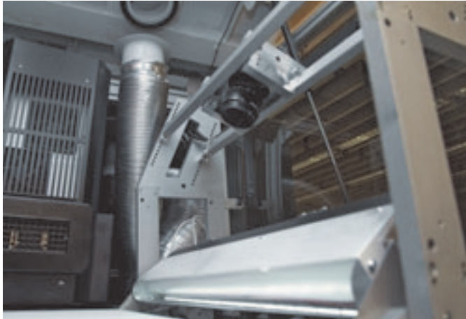
For quality assurance purposes, the VL 2000 und VL 6000 by Kodak are equipped with the Hunkeler Web Inspection System. The camera system is integrated into the printers.
