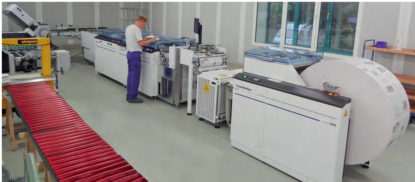
The important means for a successful business model: Halewijn uses two digital printing and Hunkeler finishing systems to produce regionalised and personalised newspapers and magazines in runs up to a single copy.
