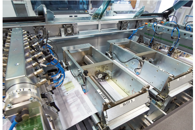
On a DP8-II Dynamic Perforating Module the individual pages are being enhanced dynamically with variable perforating patterns, both lengthwise and crosswise.
