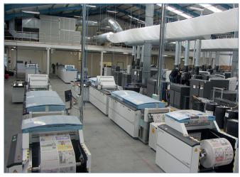
KP Services consciously opted for a production system with an offline configuration. In the event of an interruption on a printing system or finishing line, continued production is guaranteed.
