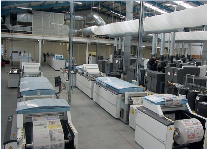
**KP Services consciously opted for a production system with an offline configuration. In the event of an interruption on a printing system or finishing line, continued production is guaranteed.**
