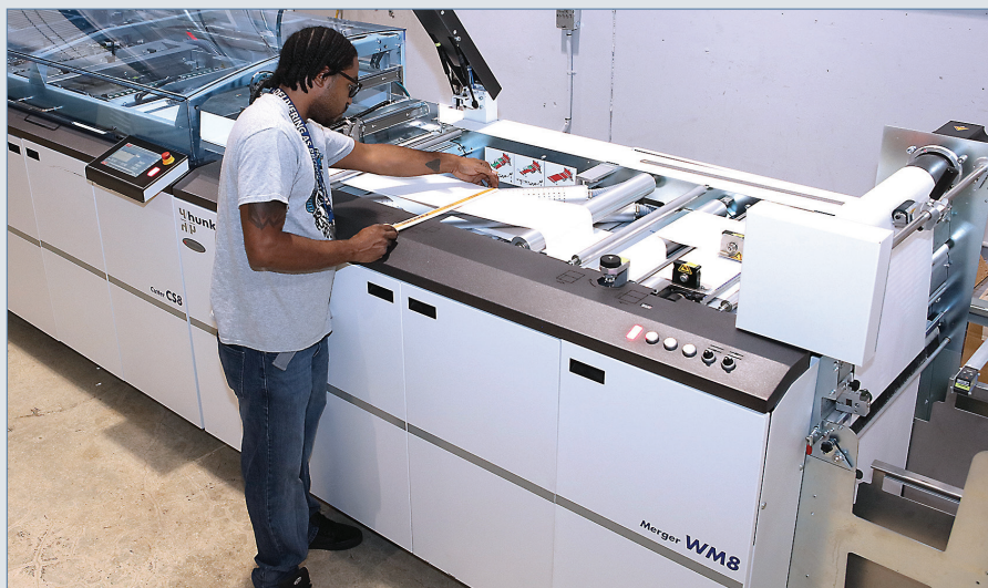
The new Hunkeler line includes the WM8 Web Merger which allows slitting and merging left under right or right under left.
