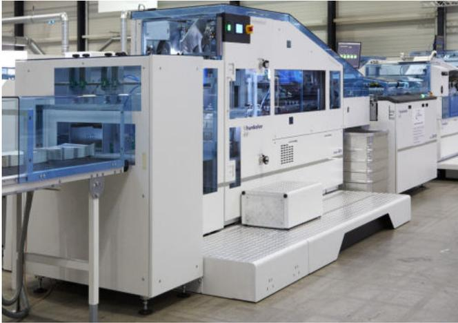
The Standard Hunkeler Roll-to-Plowfold solution at BR Printers produces ready-to-bind, glued book blocks and allows the in-line HP T240 PageWide Web press to run at its maximum rated speed.
