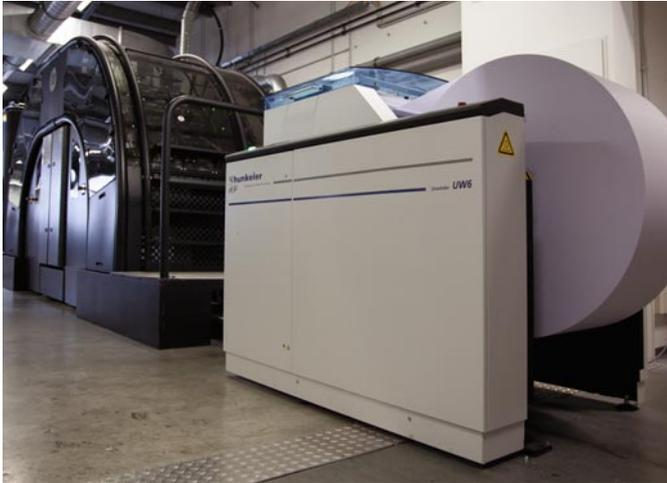
During peak times, the Hunkeler technology of the HP T200 Inkjet Web Press delivers paper 18 hours a day, with production reaching speeds between 61 and 122 meters per minute.
