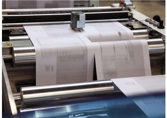
A key component in the POPP6 line is the web merger WM6. Following the slitter section, the two paper webs are precisely superimposed before they enter the CS6 cross cutter.
